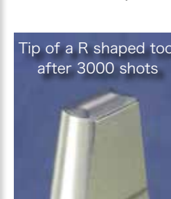
[Bonding with a R shaped tool for CIB]
