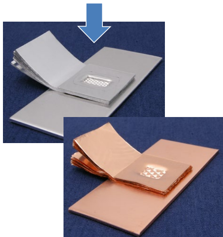
[Beautiful direct bonding of multi-foil such as <Aluminum foil and Copper foil> at once without contamination]
