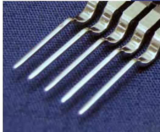
[Dipped the terminals in vibrating solder bath without flux]
